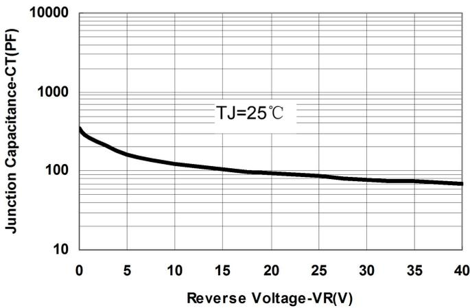
Fig.1-Typical Junction Capacitance
