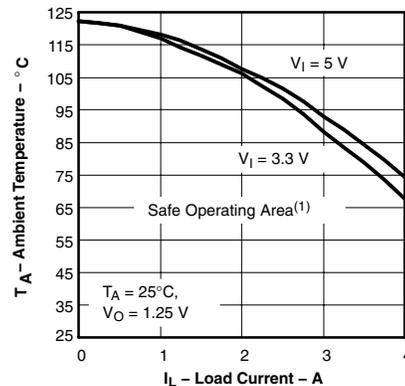
(1) Safe operating area is applicable to the test board conditions listed in the dissipation rating table section of this data sheet.
