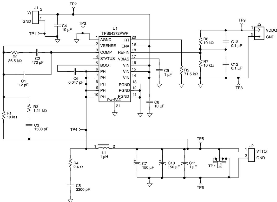
**Figure 8. Application Circuit**
