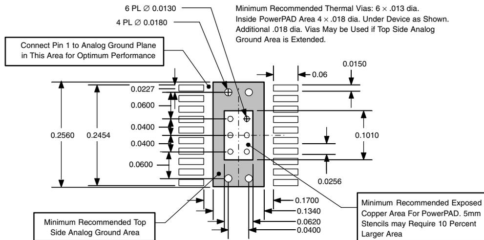
**Figure 9. Recommended Land Pattern for 20-Pin PWP PowerPAD**
