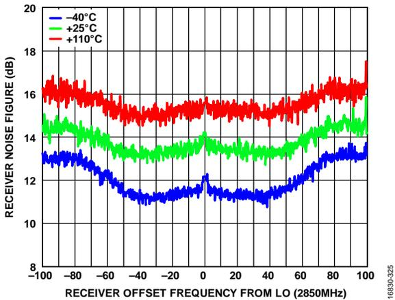
Figure 61. Receiver Noise Figure vs. Receiver Offset Frequency from LO, Integration Bandwidth = 200 kHz, LO = 2850 MHz
