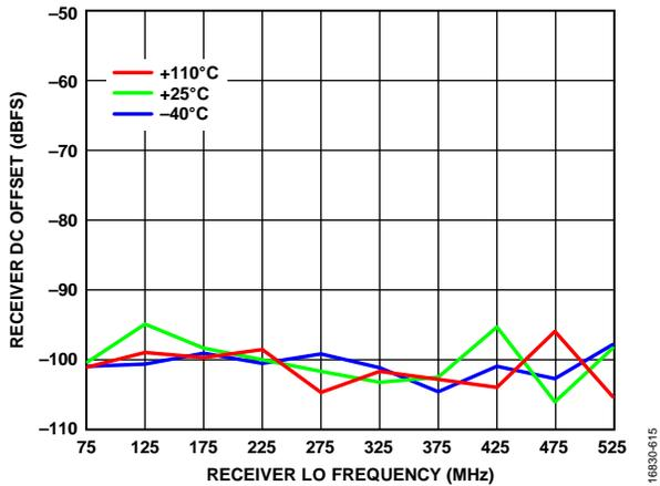
Figure 37. Receiver DC Offset vs. Receiver LO Frequency
