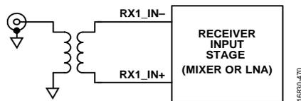
Figure 187. Differential Receiver Interface Using a Transformer
