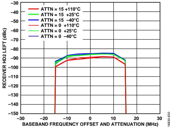
Figure 42. Receiver HD2 Left vs. Baseband Frequency Offset and Attenuation, Tone Level  $-21$  dBm at Attenuation =  $0$  dB, X-Axis Is Baseband Frequency Offset of Fundamental Tone, Not Frequency of HD2 Product (HD2 Product Is  $2 \times$  Baseband Frequency), HD2 Canceller Disabled, LO =  $525$  MHz
