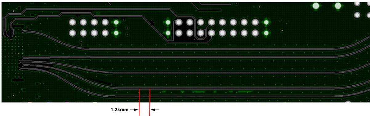
Figure 182. Via Fencing Around JESD204B Lines, PCB Layer 10
