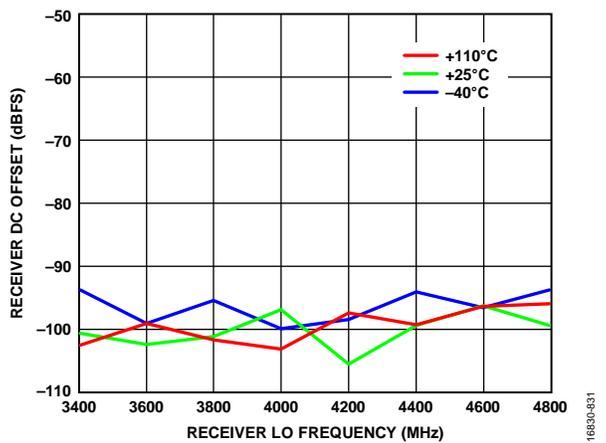
Figure 130. Receiver DC Offset vs. Receiver LO Frequency
