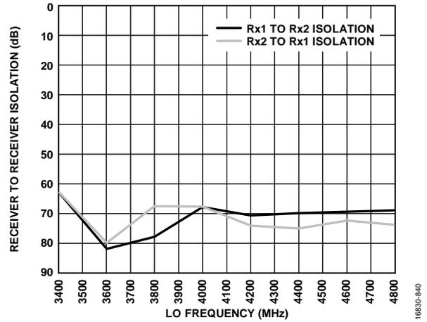
Figure 139. Receiver to Receiver Isolation vs. LO Frequency
