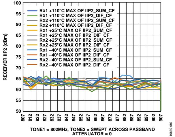
Figure 68. Receiver IIP2 Sum and Difference Across Bandwidth, Receiver Attenuation = 0 dB, LO = 800 MHz, Tone 1 = 802 MHz, Tone 2 Swept, -21 dBm Each, IIP2\_SUM\_CF and IIP2\_DIF\_CF Indicate Sum and Difference Products
