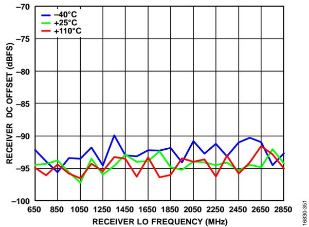
Figure 87. Receiver DC Offset vs. Receiver LO Frequency
