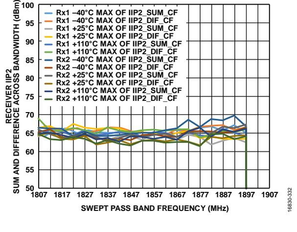
Figure 69. Receiver IIP2 Sum and Difference Across Bandwidth vs. Swept Pass Band Frequency, Receiver Attenuation = 0 dB, LO = 1800 MHz, Tone 1 = 1802 MHz, Tone 2 Swept, -21 dBm Each, IIP2\_SUM\_CF and IIP2\_DIF\_CF Indicate Sum and Difference Products
