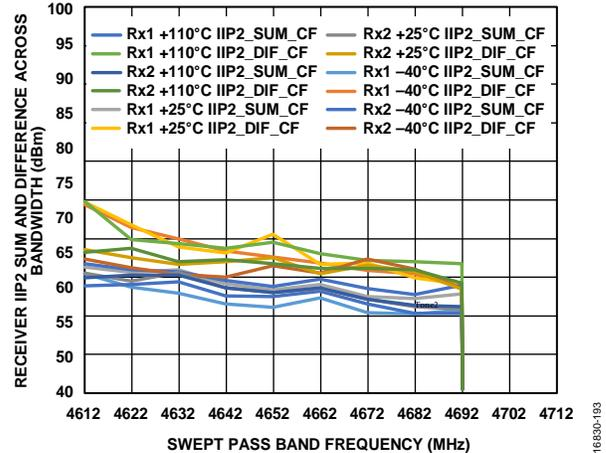
Figure 112. Receiver IIP2 Sum and Difference Across Bandwidth vs. Swept Pass Band Frequency, Receiver Attenuation = 0 dB, LO = 4600 MHz, Tone 1 = 4602 MHz, Tone 2 Swept, -21 dBm Each, IIP2\_SUM\_CF and IIP2\_DIF\_CF Indicate Sum and Difference Products
