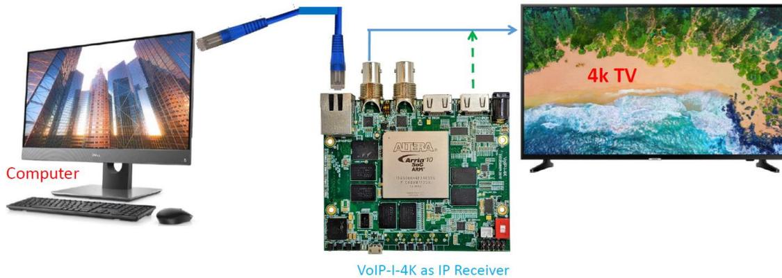
Fig. 6 Setup for evaluating the SOC decoder IP core using a computer and one VoIP-I-4K
