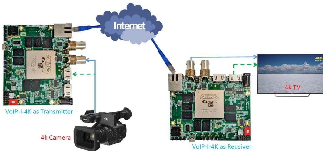
Fig. 3 The VoIP-I-4K is used for 4K video-over-IP
