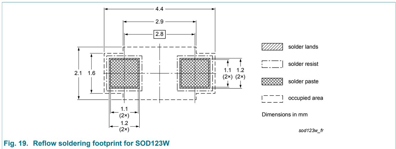
Fig. 19. Reflow soldering footprint for SOD123W
