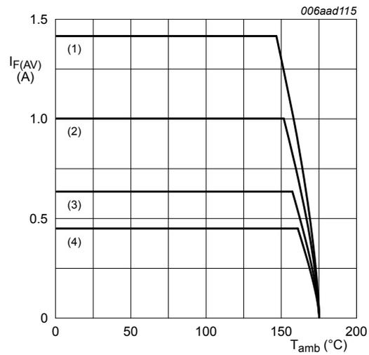
Ceramic PCB,  $\text{Al}_2\text{O}_3$ , standard footprint
