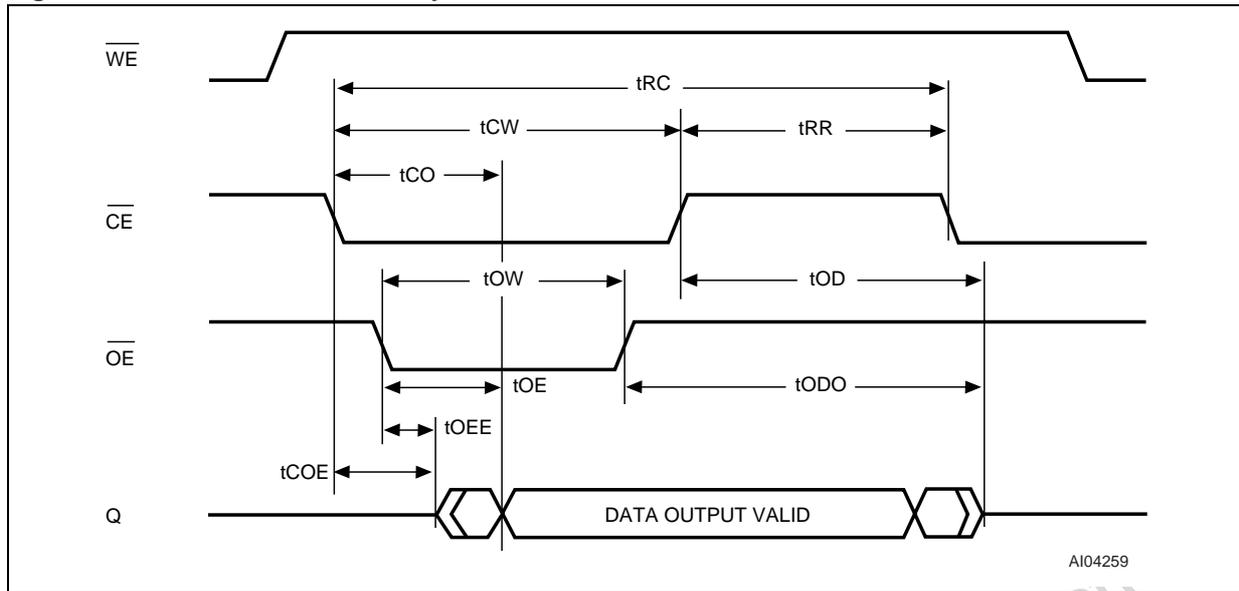
Figure 10. Phantom Clock WRITE Cycle
