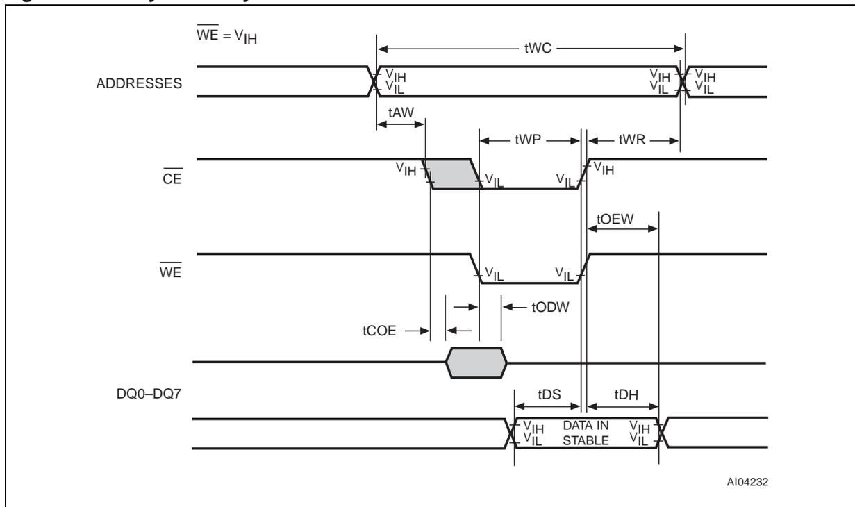
Note: 1.  $\overline{OE} = V_{IH}$  or  $V_{IL}$ . If  $\overline{OE} = V_{IH}$  during a WRITE cycle, the output buffers remain in a high impedance state.
