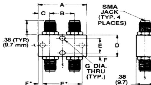
All dimensions are  $\pm .020$  except mounting diameters ( $\pm .005$ ) and mounting hole location ( $\pm .010$ ).
