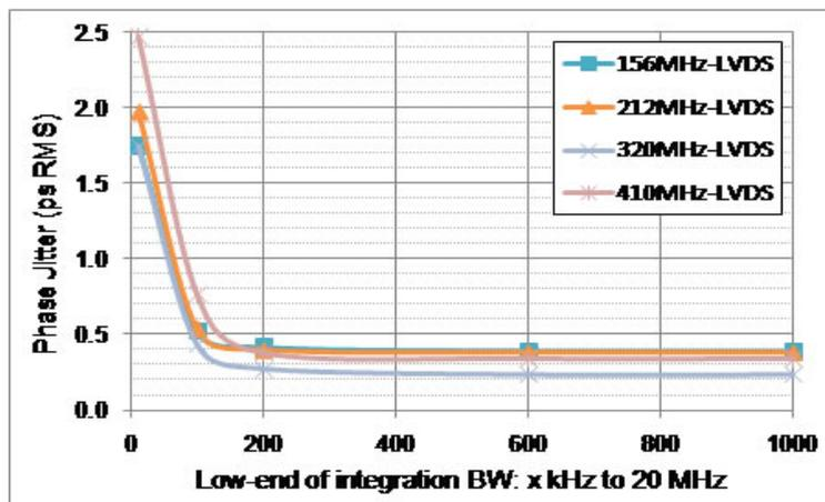
Figure 2. LVDS Phase Jitter (integrated phase noise)
