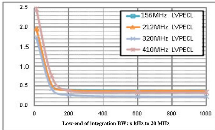
Figure 1. LVPECL Phase Jitter (integrated phase noise)
