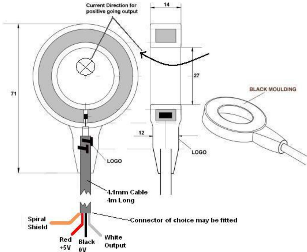
**NB:** For best accuracy centre primary conductor in aperture
