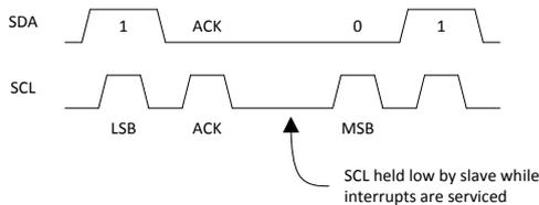
Figure 6, Clock stretching
