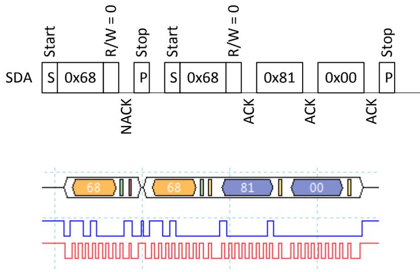
2 Write calibration target 500 to register Calibration Target (0x84)
