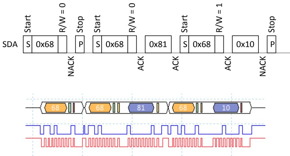
Calibration status register = 0x10 means target calibration succeeded.
