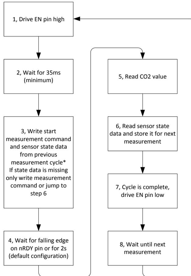
\*If start measurement command and state data is written in two separate write sequences, state data must be written before start measurement command
