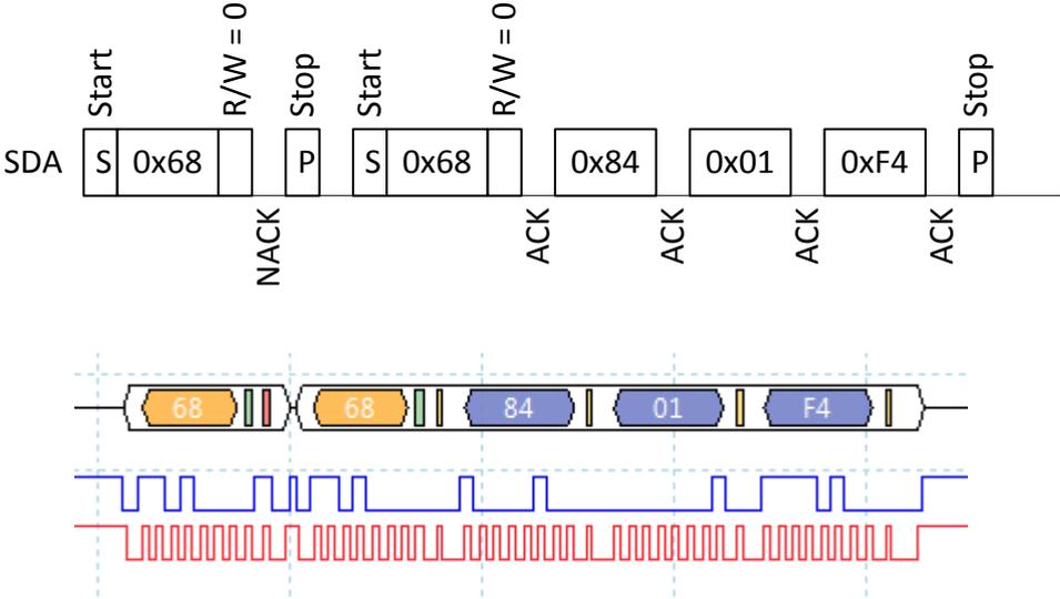
3 Write calibration command (0x7C05) to register Calibration Command (0x82)
