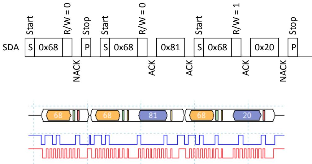
Calibration status register = 0x20 means background calibration succeeded.
