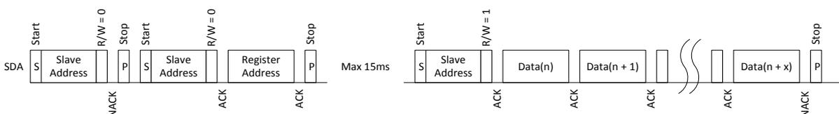
Figure 7, Reading from Senseair Sunrise after wake up
