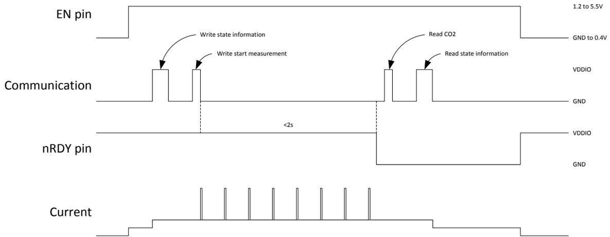
**Figure 11, Timing diagram for single measurement mode**
