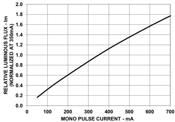
Figure 6: Relative Radiant Flux vs. Mono Pulse Current for Far Red, Deep Red, and Royal Blue
