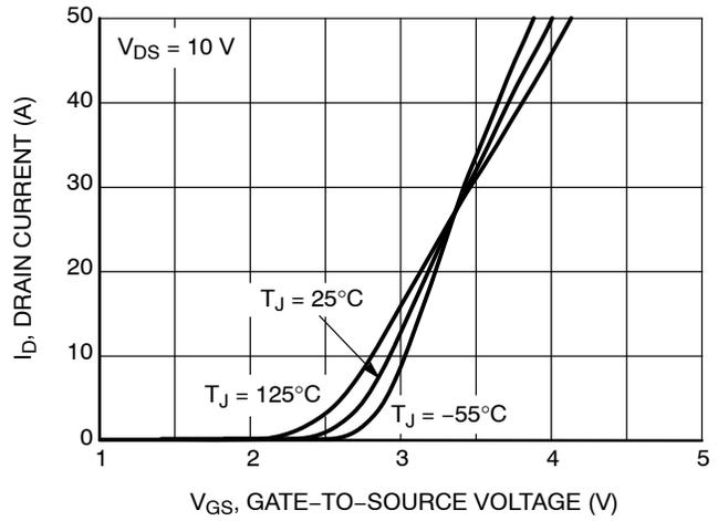
Figure 2. Transfer Characteristics
