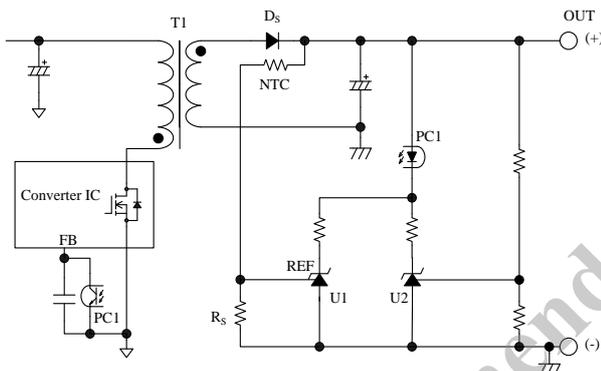
Figure 6-1 Reference temperature detection circuit with NTC thermistor
