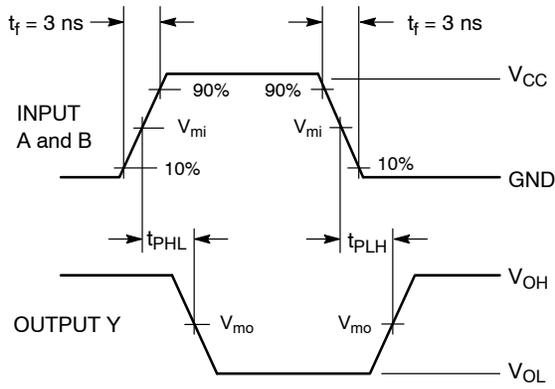
**Figure 3. Switching Waveform**
