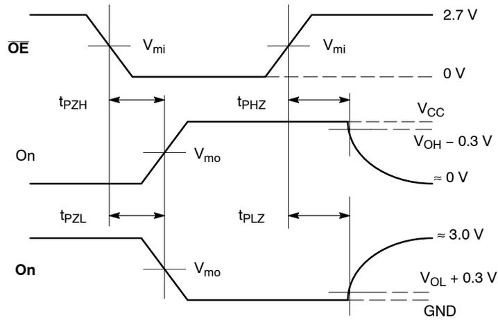
**Figure 7. AC Output Enable and Disable Waveform**
