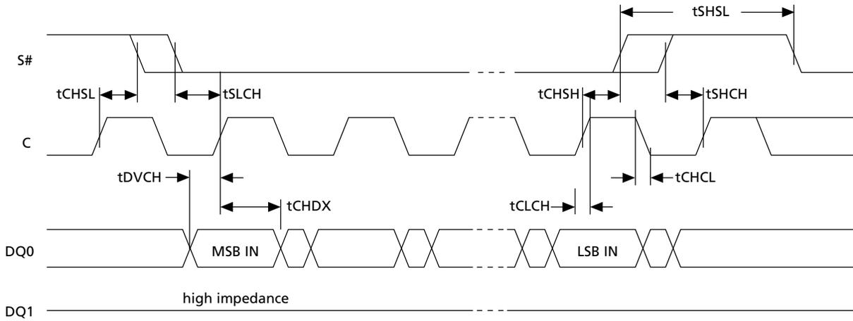
**Figure 22: Write Protect Setup and Hold during WRSR when SRWD=1 Timing**
