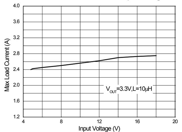
**Performance Characteristics** (continued) ( $T_A=+25^{\circ}\text{C}$ ,  $V_{IN}=12\text{V}$ ,  $V_{OUT}=3.3\text{V}$ , unless otherwise noted.)
