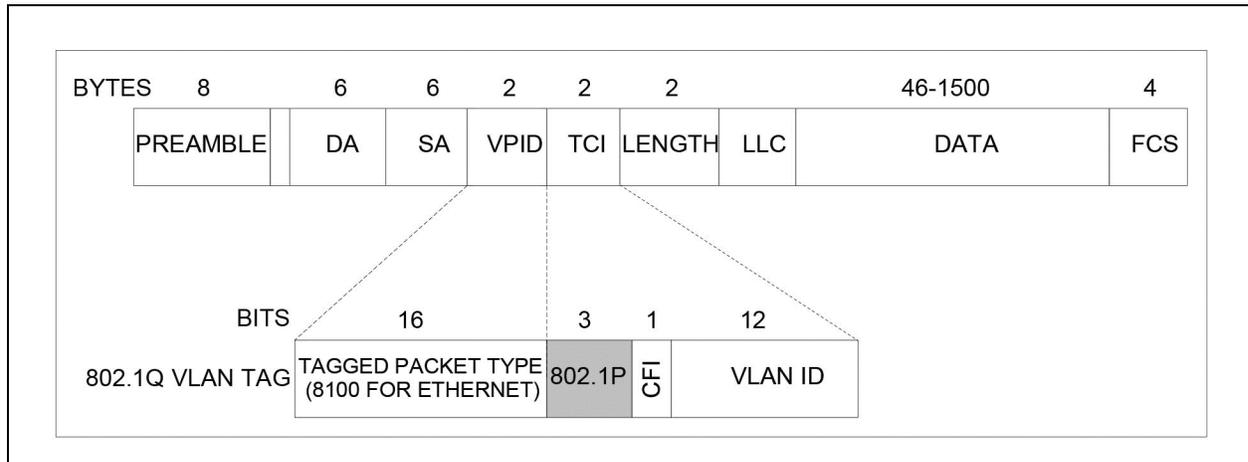
The 802.1p-based priority is enabled by Bit[5] of the Port Control 0 Registers for ports 1, 2, 3, 4 and 5, respectively.
