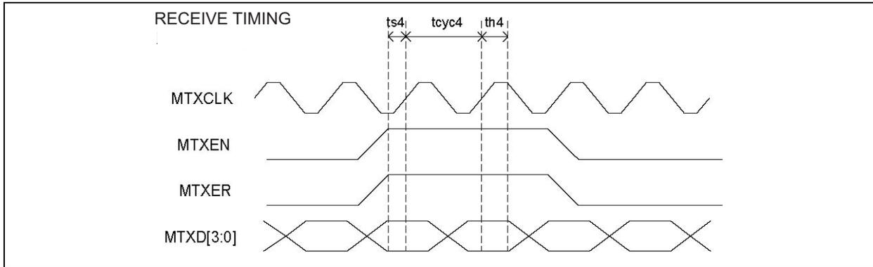
**FIGURE 7-6: PHY MODE MII TIMING - DATA TRANSMITTED FROM MII**
