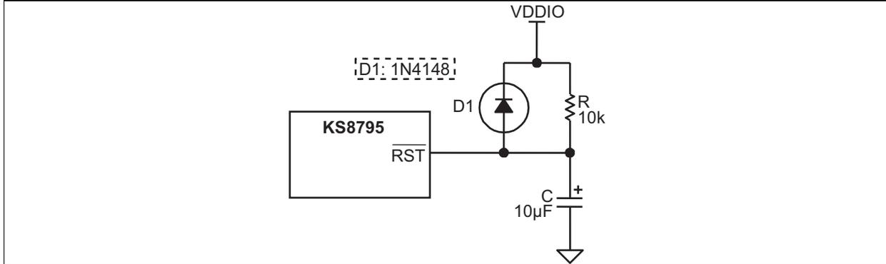
**FIGURE 8-2: RECOMMENDED CIRCUIT FOR INTERFACING WITH CPU/FPGA RESET**
