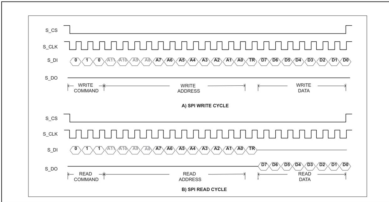
**FIGURE 3-8: SPI MULTIPLE ACCESS TIMING**
