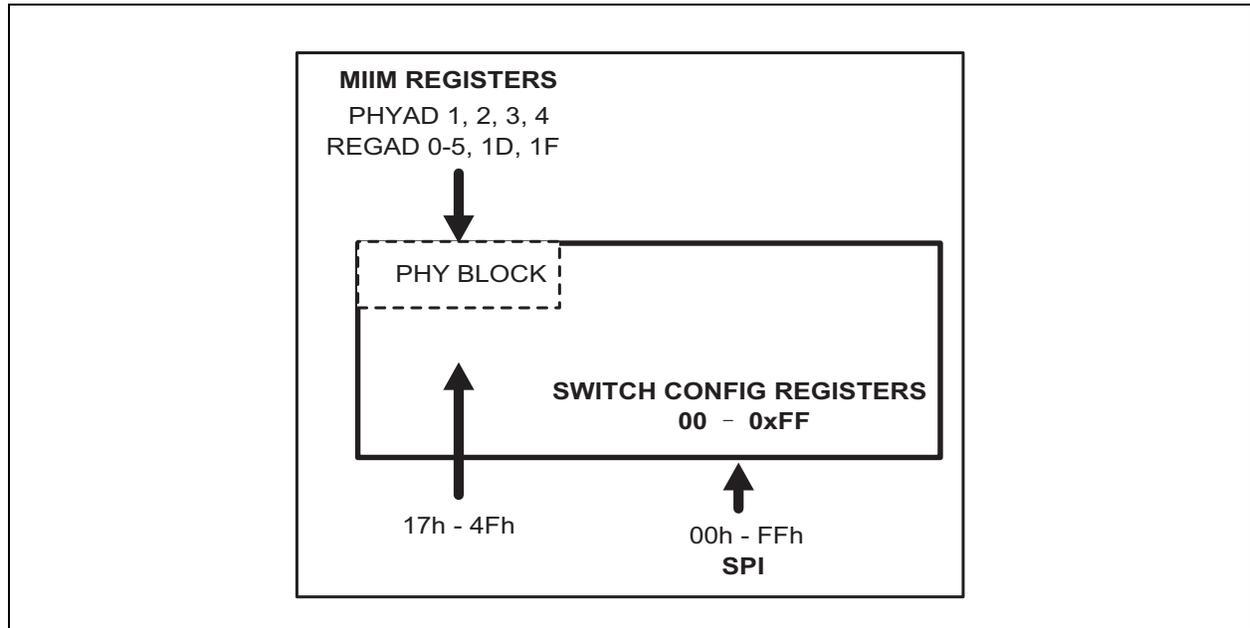
The registers within the linear 0x00-0xFF address space are all accessible via the SPI interface by a CPU attached to that bus. The mapping of the various functions within that linear address space is summarized in [Table 4-1](#).
