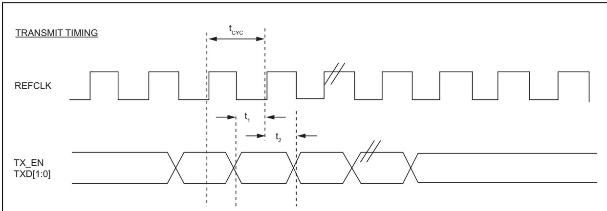
**FIGURE 7-8: RMII TIMING - DATA TRANSMITTED FROM RMII**
