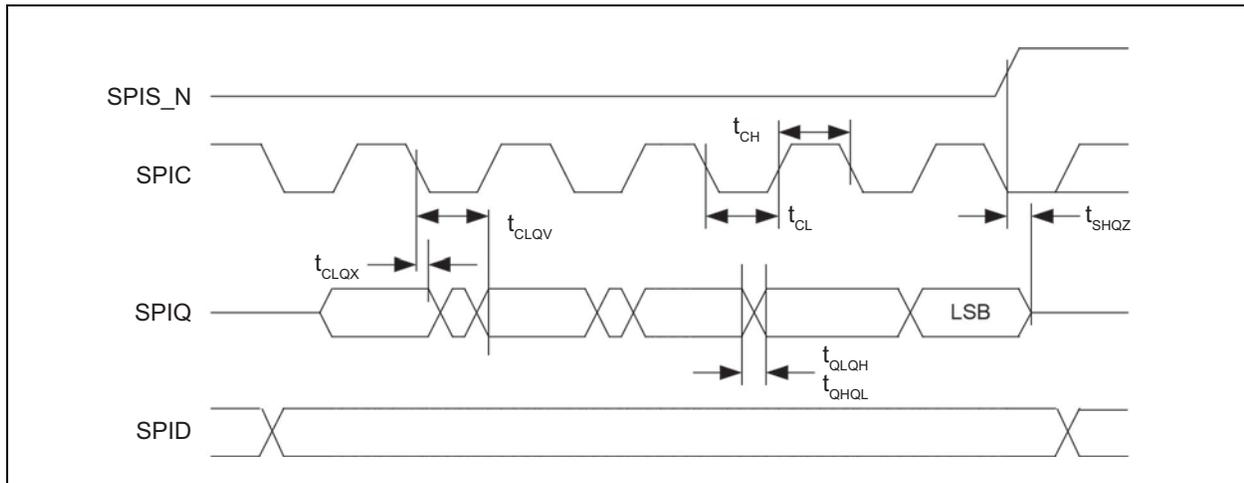
**TABLE 7-7: SPI OUTPUT TIMING PARAMETERS**
