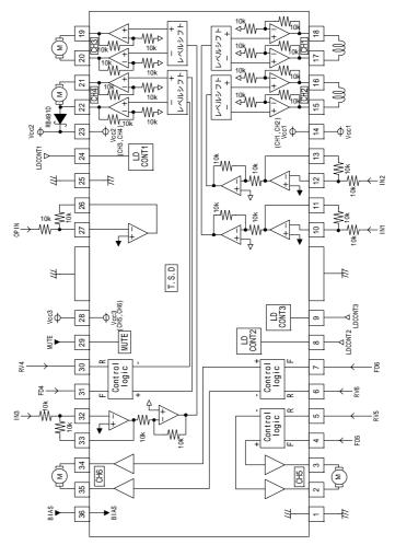
T.S.D: (Thermal shutdown) Resistance unit :  $[\Omega]$
