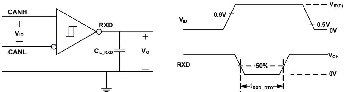
Figure 2. RXD Dominant Timeout Test Circuit and Measurement
