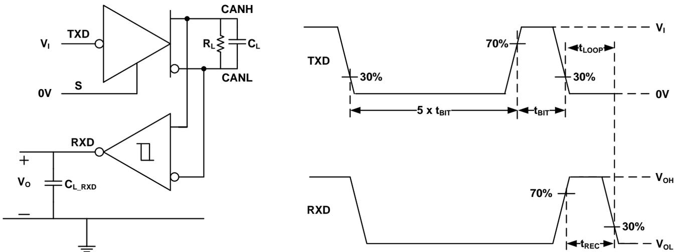
Note:  $t_{LOOP}$  is equivalent to  $t_{PROP(LOOP)}$  from CAN timing.
