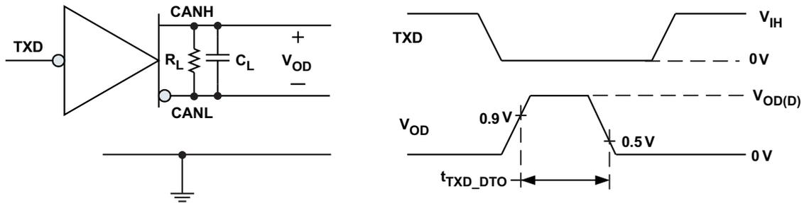
**Figure 9. TXD Dominant Timeout Test Circuit and Measurement**
