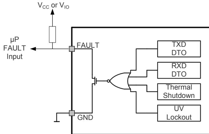
Figure 11. FAULT Terminal Function Diagram and Application
