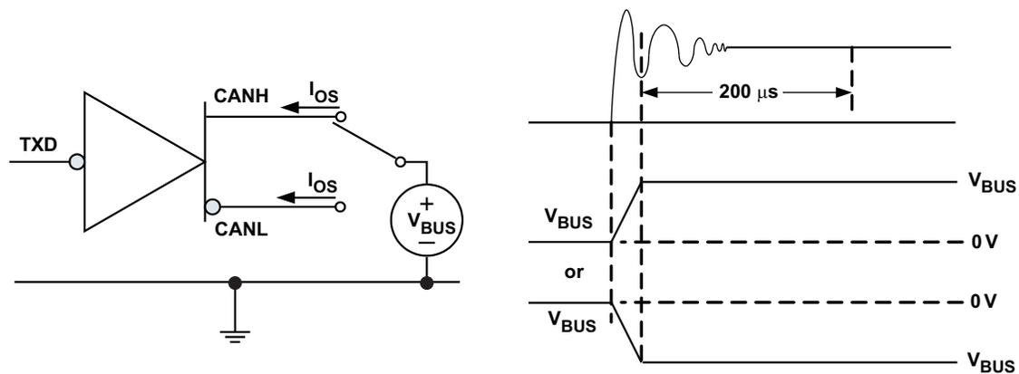
**Figure 10. Driver Short Circuit Current Test and Measurement**
