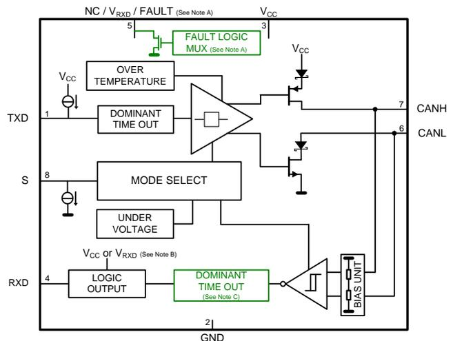
Terminal 5 function is device dependent; NC on SN65HVD265,  $V_{RXD}$  for RXD output level-shifting device on SN65HVD266, and FAULT Output on SN65HVD267
