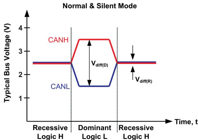
**Figure 14. Bus States (Physical Bit Representation)**
