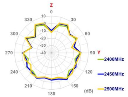
3-D Radiation Pattern on 30cm\*30cm Ground Plane @2450MHz
