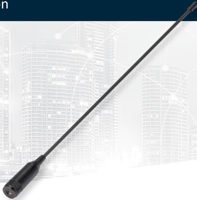
The FW.24 is a flexible 2.4GHz whip antenna with a SMA(M) connector for outdoor use. It features excellent efficiency (>75%) and high peak gain (>4 dBi) between 2400-2500MHz on a 30\*30cm ground plane.
