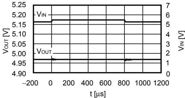
2. Characteristics of load transient response (Ta = +25°C)
