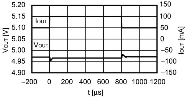
$V_{IN} = 5.5\text{ V}$ ,  $C_{OUT} = 4.7\ \mu\text{F}$ ,  $C_{IN} = 4.7\ \mu\text{F}$ ,  $I_{OUT} = 100\text{ mA} \leftrightarrow 500\text{ mA}$
