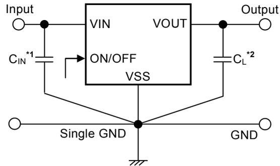
\*1.  $C_{IN}$  is a capacitor for stabilizing the input.
