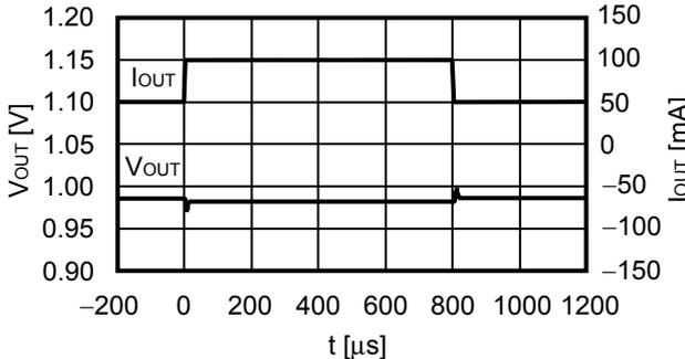
$V_{IN} = 2.0\text{ V}$ ,  $C_{OUT} = 4.7\ \mu\text{F}$ ,  $C_{IN} = 4.7\ \mu\text{F}$ ,  $I_{OUT} = 100\text{ mA} \leftrightarrow 500\text{ mA}$
