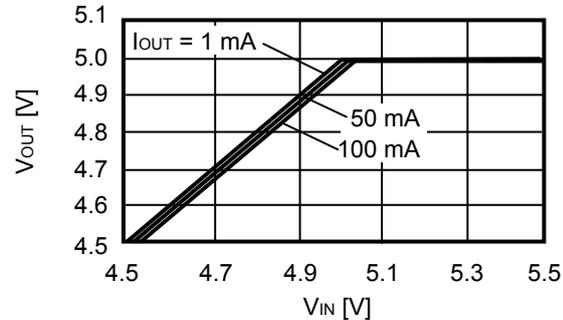
**3. Dropout voltage vs. Output current**
