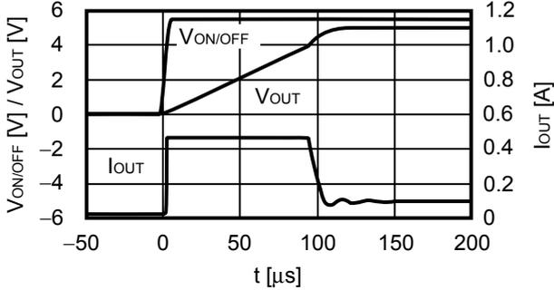
V<sub>IN</sub> = 5.5 V, C<sub>OUT</sub> = 4.7 μF, C<sub>IN</sub> = 4.7 μF, I<sub>OUT</sub> = 1000 mA
