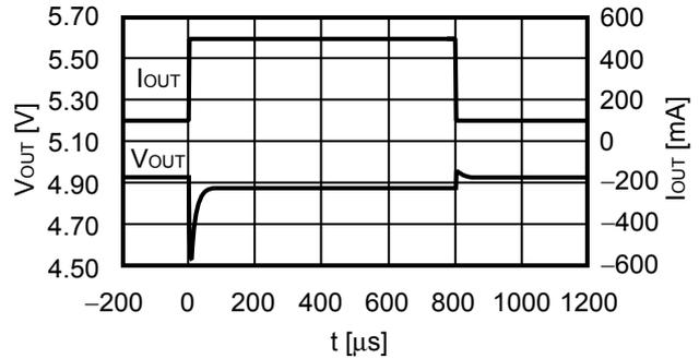
3. Transient response characteristics of ON/OFF pin ( $T_a = +25^\circ\text{C}$ )
