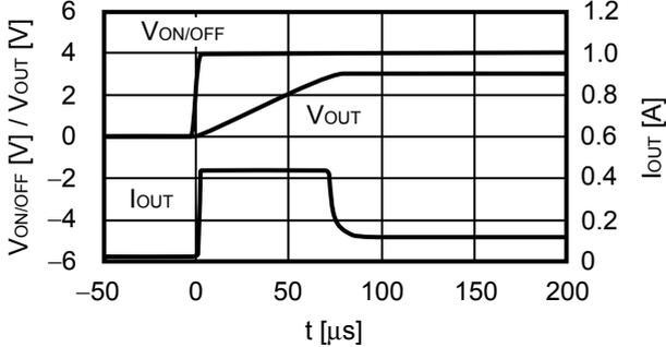
V<sub>IN</sub> = 4.0 V, C<sub>OUT</sub> = 4.7 μF, C<sub>IN</sub> = 4.7 μF, I<sub>OUT</sub> = 1000 mA
