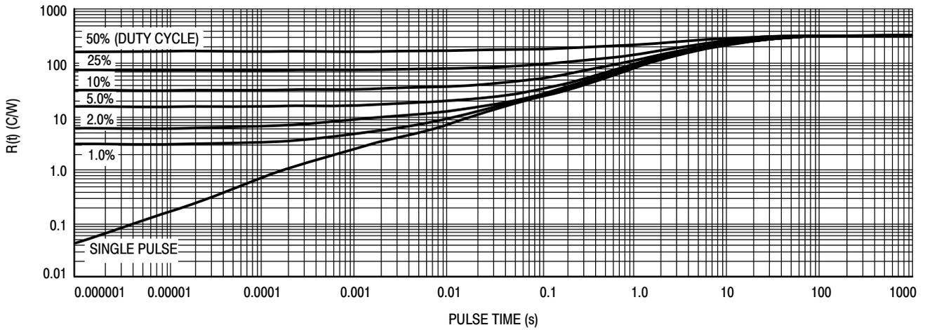
Figure 8. Thermal Response, Junction-to-Ambient ( $20\text{ mm}^2$  pad)
