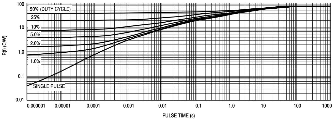
Figure 9. Thermal Response, Junction-to-Ambient ( $1\text{ in}^2$  pad)
