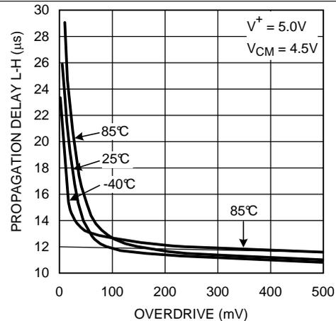
Figure 18. Propagation Delay vs Overdrive
