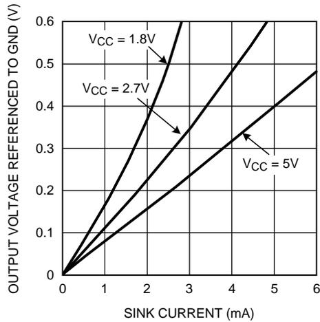
Figure 7. Output Voltage Low vs Sink Current
