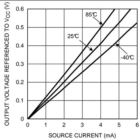
Figure 10. Output Voltage High vs Source Current
