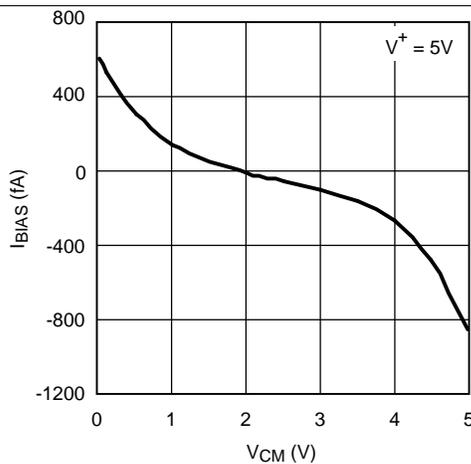
Figure 23.  $I_{BIAS}$  vs  $V_{CM}$
