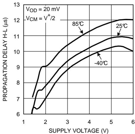
Figure 11. Propagation Delay vs Supply Voltage
