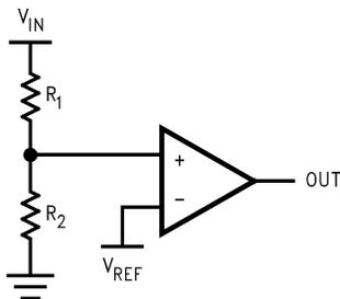
Figure 36. Threshold Detector
