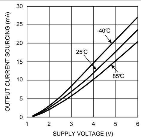
Figure 6. Short-Circuit Sourcing Current vs Supply Voltage
