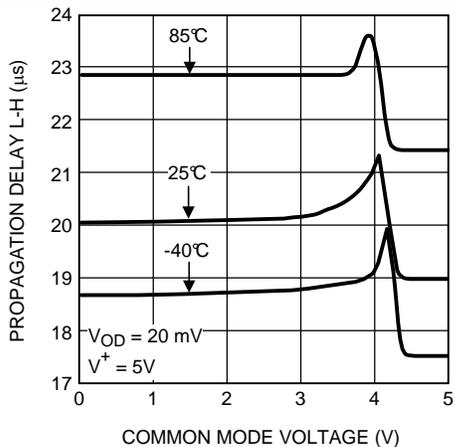
Figure 27. Propagation Delay vs Common-Mode Input
