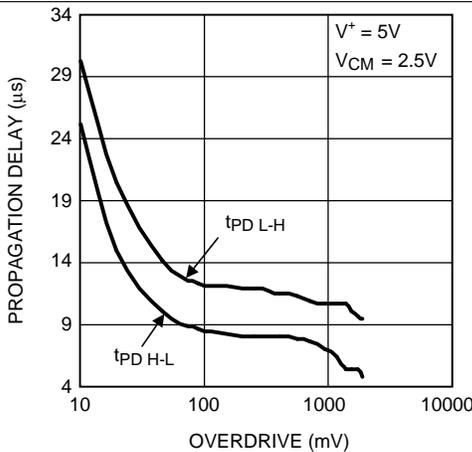
Figure 17. Propagation Delay vs Overdrive
