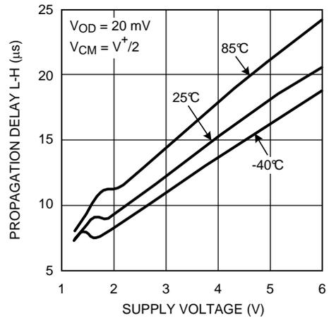
Figure 12. Propagation Delay vs Supply Voltage
