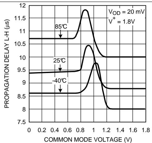
Figure 24. Propagation Delay vs Common-Mode Input
