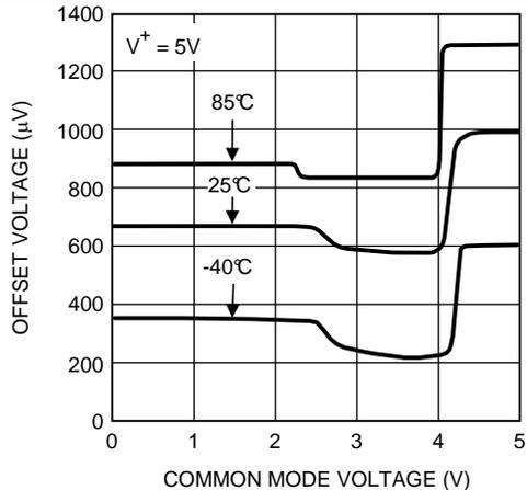
Figure 28. Offset Voltage vs Common-Mode Input
