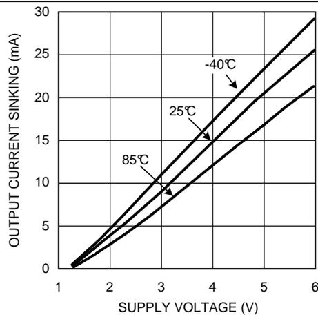
Figure 5. Short-Circuit Sinking Current vs Supply Voltage
