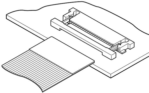
**Compact connector with just 1.2mm high after mounting on the PC board.**
