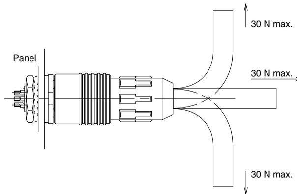
2. To maintain the water/dust protection performance and the cable clamp force, use a cable that is within the range of applicable cable diameter.
