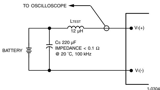
Note: Input reflected-ripple current is measured with a simulated source impedance of 12  $\mu$ H. Capacitor Cs offsets possible battery impedance. Current is measured at the input of the module.
