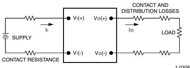
Note: All measurements are taken at the module terminals. When socketing, place Kelvin connections at module terminals to avoid measurement errors due to socket contact resistance.
