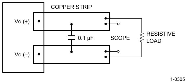
Note: Use a 0.1  $\mu$ F ceramic capacitor. Scope measurement should be made using a BNC socket. Position the load between 50.8 mm and 76.2 mm (2 in. and 3 in.) from the module.
