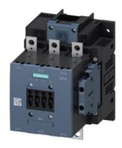
power contactor, AC-3 115 A, 55 kW / 400 V AC (50-60 Hz) / DC operation 220-240 V AC/DC auxiliary contacts 2 NO + 2 NC 3-pole, frame size S6 busbar connections drive: conventional screw terminal
