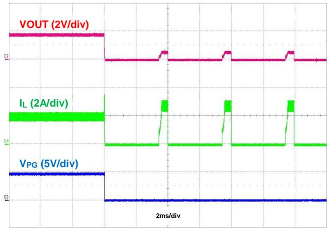
Figure 39. Output Short Protection, IOU = 2A
