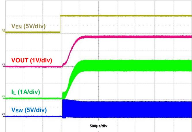
Figure 33. Startup Using EN, IOUT = 2A
