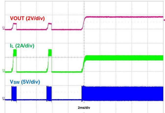
Figure 36. Output Short Recovery, IOUT = 2A
