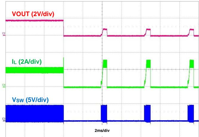
Figure 35. Output Short Protection, IOUT = 2A
