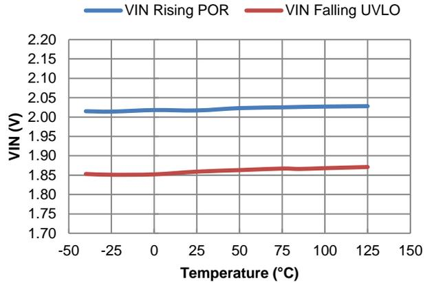
Figure 9.  $V_{IN}$  Power-On Reset and UVLO vs. Temperature
