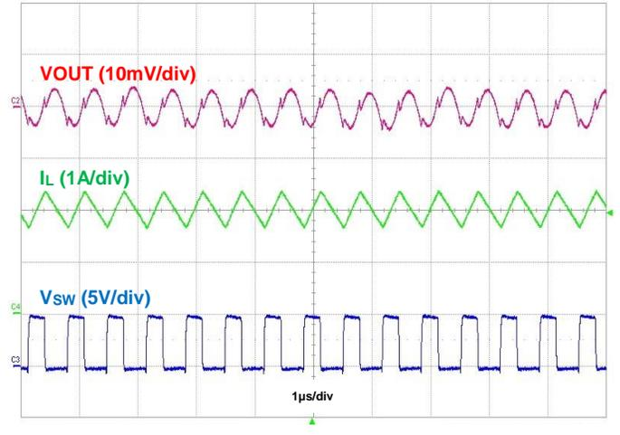
Figure 17. Output Voltage Ripple, IOUT = 2A
