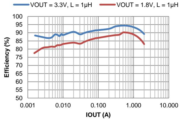
Figure 11. Efficiency vs. Output Current,  $V_{IN} = 5\text{V}$
