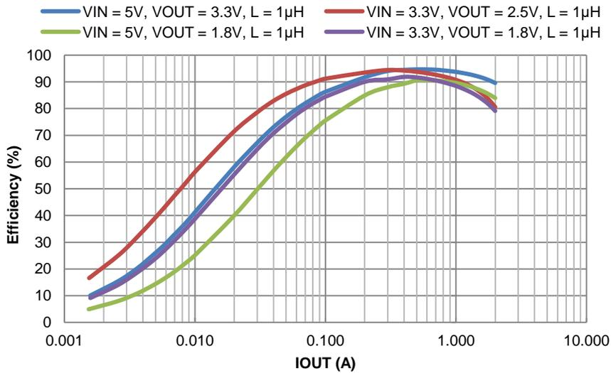
Figure 4. PWM Efficiency vs. Output Current
