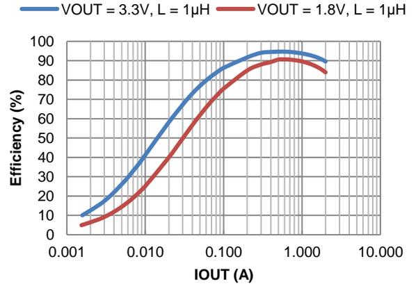
Figure 22. Efficiency vs. Output Current,  $V_{IN} = 5\text{V}$
