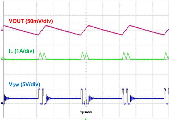
Figure 16. Output Voltage Ripple, IOUT = 50mA
