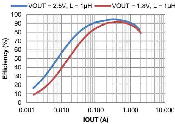
Figure 21. Efficiency vs. Output Current,  $V_{IN} = 3.3\text{V}$
