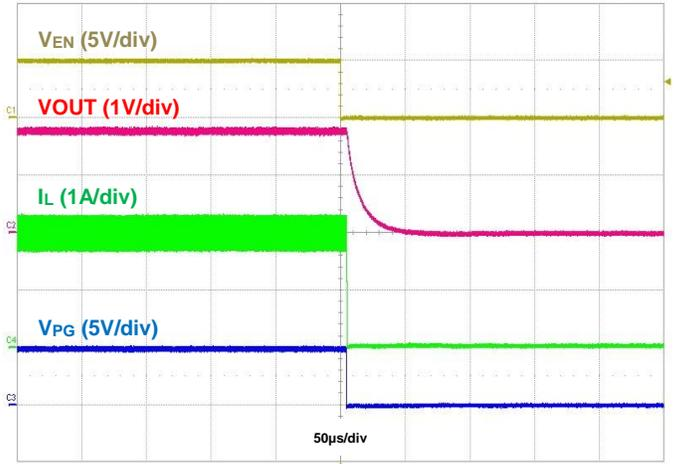
Figure 38. Shutdown Using EN, IOU = 2A
