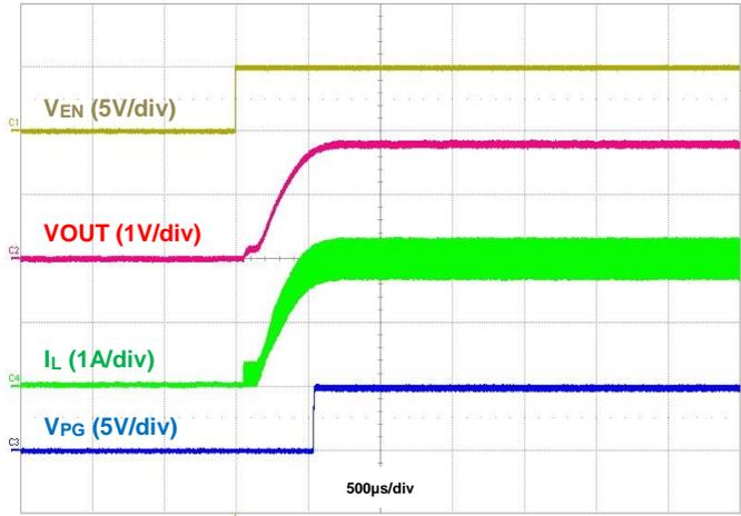
Figure 37. Startup Using EN, IOU = 2A
