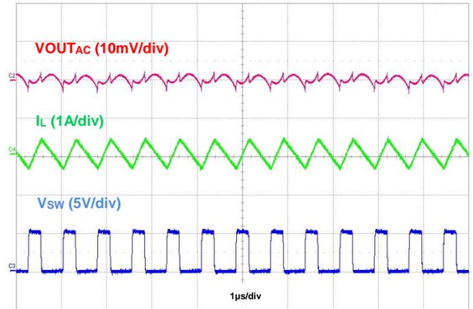
Figure 28. Output Voltage Ripple, IOUt = 50mA
