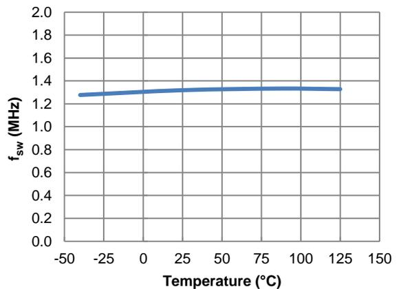
Figure 26.  $f_{sw}$  vs. Temperature,  $I_{OUT} = 0\text{A}$
