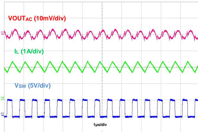
Figure 29. Output Voltage Ripple, IOUt = 2A
