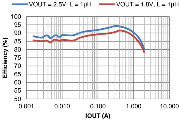
Figure 10. Efficiency vs. Output Current,  $V_{IN} = 3.3\text{V}$
