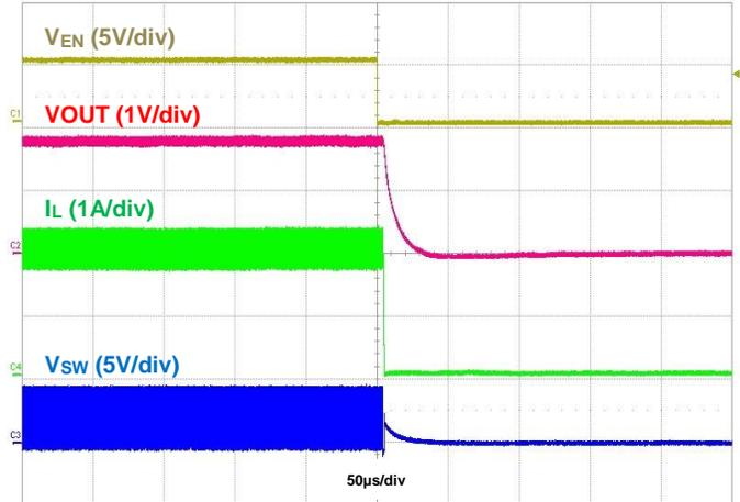
Figure 34. Shutdown Using EN, IOUT = 2A
