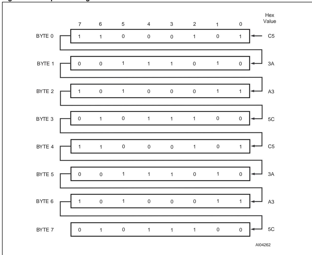
Note: The odds of this pattern being accidentally duplicated and sending aberrant entries to the RTC is less than 1 in  $10^{19}$ . This pattern is sent to the clock LSB to MSB.
