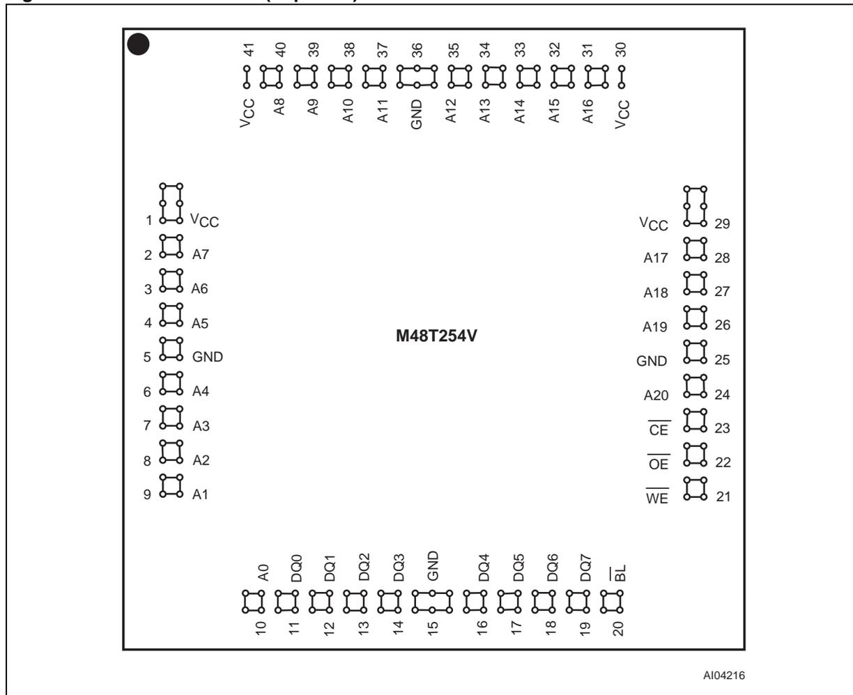
Note: This diagram is TOP VIEW perspective (view through package).
