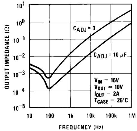
Figure 8. Output Impedance
