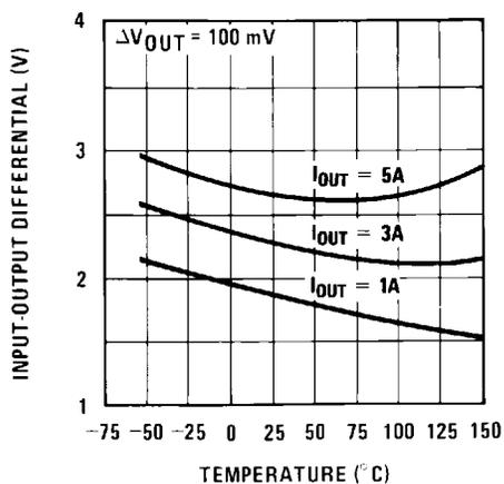
Figure 5. Dropout Voltage
