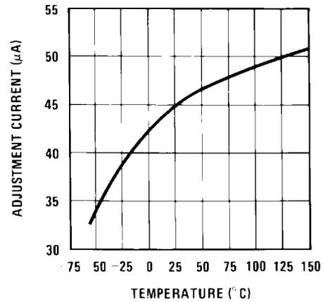
Figure 6. Adjustment Current
