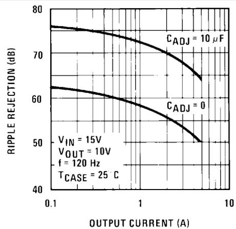
Figure 12. Ripple Rejection
