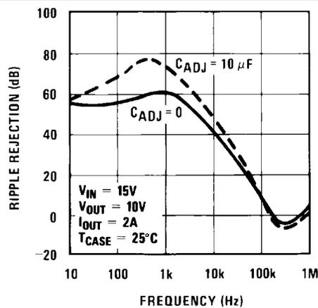
Figure 11. Ripple Rejection
