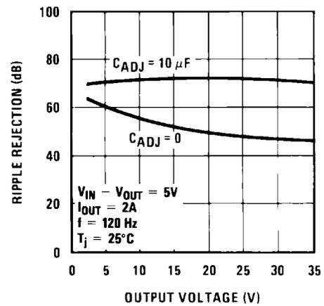
Figure 10. Ripple Rejection
