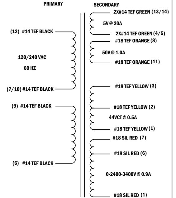
PIN NUMBERS FOR EACH CONNECTOR ARE INDICATED IN BRACKETS
