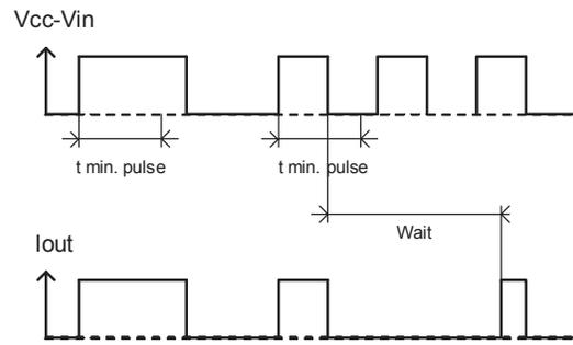
**Figure 4 – Min. pulse and Wait function**
