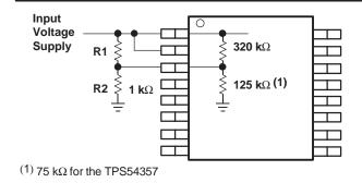
Figure 1. Circuit Using External UVLO Function
