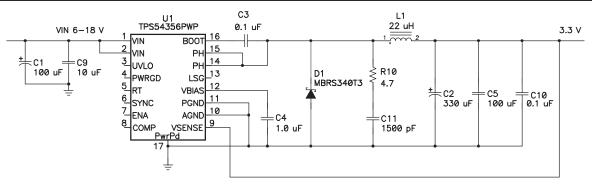
Figure 26. 3.3-V Power Supply With Schottky Diode
