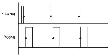
Figure 3. SYNC Input Waveform
