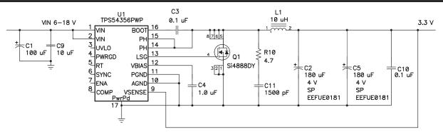
Figure 29. 3.3-V Power Supply with Panasonic SP Output Filter Capacitors
