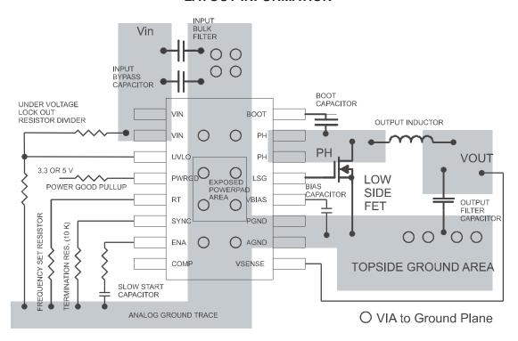
Figure 23. TPS5435x PCB Layout
