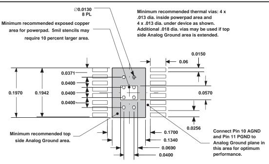
Figure 24. Thermal Considerations for PowerPAD Layout
