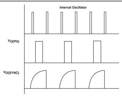
Figure 4. SYNC Output Waveform
