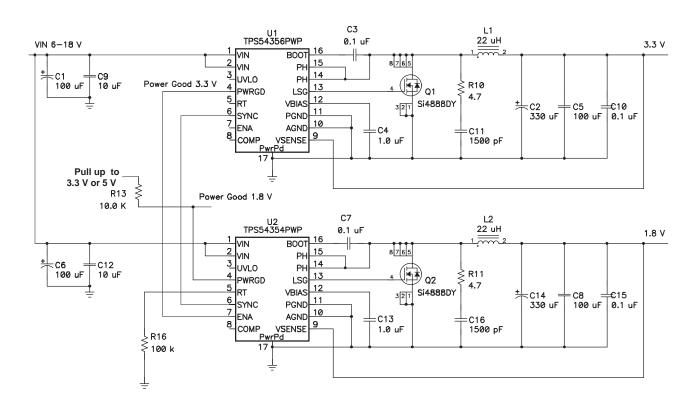
Figure 27. 3.3-V/1.8-V Power Supply with Sequencing
