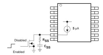
Figure 2. Interfacing to the ENA Pin
