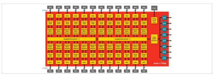
Virtex-7 FPGAs reduce size, weight, power, and cost (SWaP-C) for airborne/vehicular-based radar systems. A single board with three Virtex-7 980XT FPGAs implementing a 64-channel beamformer enables portable form factor with:
