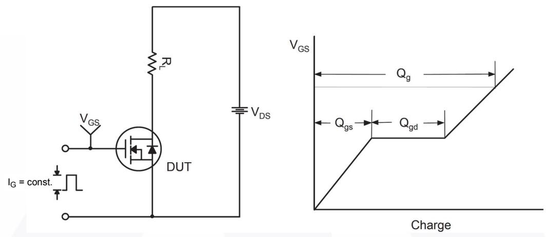
**Figure 14. Gate Charge Test Circuit & Waveform**
