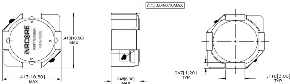
NOTE: Pin 3 and Pin 4 are for mechanical connection only.
