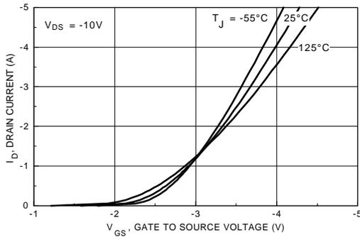
Figure 5. Transfer Characteristics.
