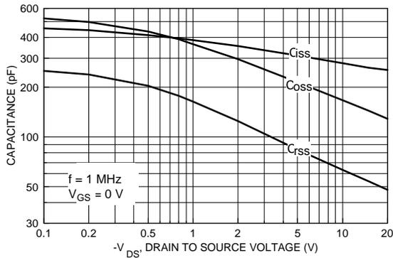
**Figure 9. Capacitance Characteristics.**
