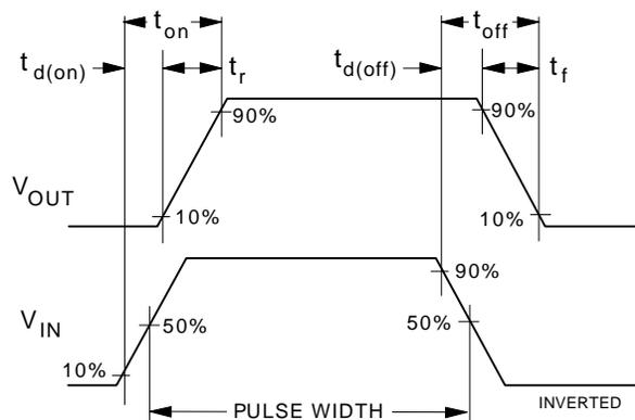
**Figure 12. Switching Waveforms.**
