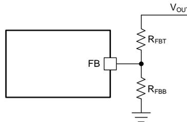
**Figure 11. Output Voltage Setting**
