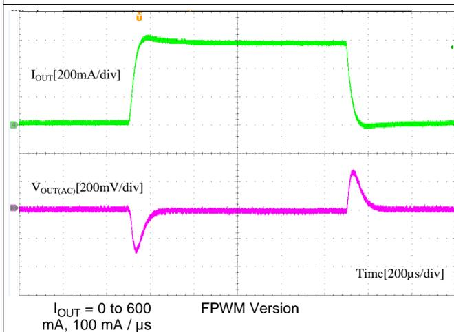
Figure 20. Load Transient
