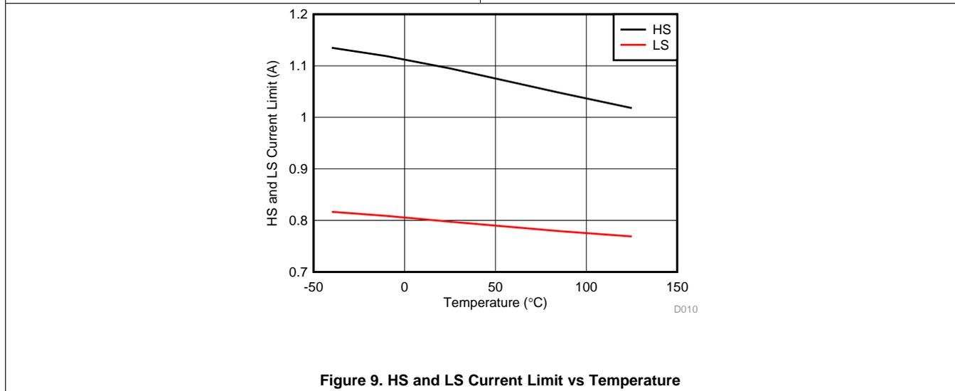
**Figure 9. HS and LS Current Limit vs Temperature**
