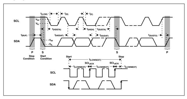
Figure 12: Example Timing Diagram for SMBus Send Byte Format
