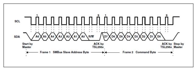
Figure 13: Example Timing Diagram for SMBus Receive Byte Format
