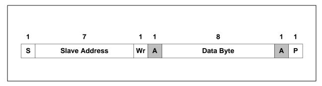
Figure 20: SMBus Receive Byte Protocol
