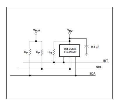
Pull-up resistors ( $R_p$ ) maintain the SDAH and SCLH lines at a *high* level when the bus is free and ensure the signals are pulled up from a low to a high level within the required rise time. For a complete description of the SMBus maximum and minimum  $R_p$  values, please review the SMBus Specification at www.smbus.org/specs. For a complete description of  $I^2C$  maximum and minimum  $R_p$  values, please review the  $I^2C$  Specification at www.nxp.com.
