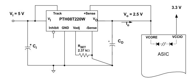
Figure 24. Application Circuit Demonstrating Prebias Startup
