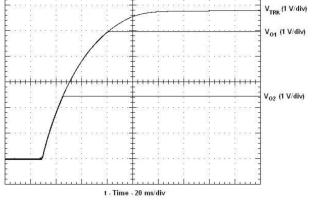
Figure 16. Simultaneous Power Up With Auto-Track Control
