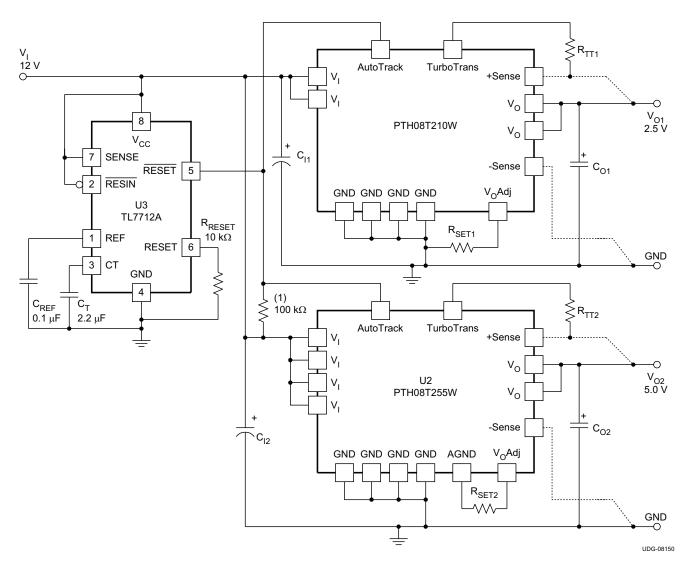
(1) When using Auto-Track with the PTH08T255W, a 100-k $\Omega$  resistor must be placed between the VI and AutoTrack pins.
