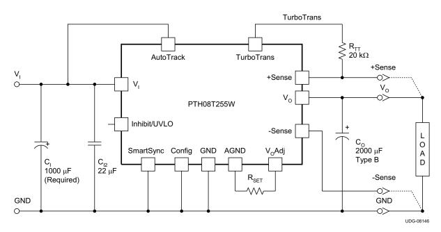
Figure 9. Typical TurboTrans™ Application
