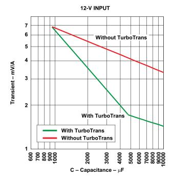
Figure 7. Capacitor Type B, 1000 < C( $\mu$ F)×ESR(m $\Omega$ ) ≤ 5000 (e.g. Polymer-Tantalum)
