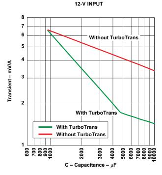
Figure 8. Capacitor Type C, 5000 < C( $\mu$ F)×ESR(m $\Omega$ ) ≤ 10,000(e.g. OS-CON)
