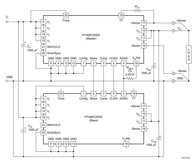
Figure 19. Typical Current Sharing Diagram
