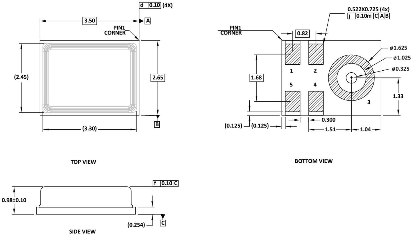
Figure 15. 5-Terminal Chip Array Small Outline No Lead Cavity [LGA\_CAV]
