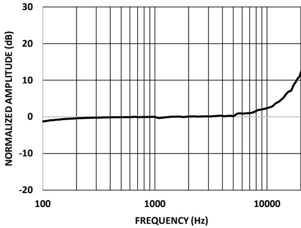
Figure 4. Typical Audio Frequency Response, Standard Mode
