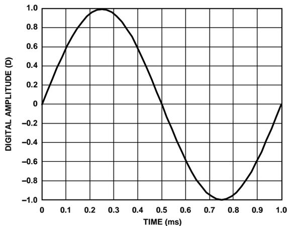
**Figure 9. 1 kHz, 0 dB FS Sine Wave**
