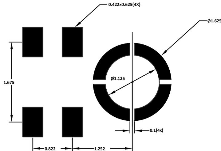
**Figure 14. Suggested Solder Paste Stencil Pattern Layout**
