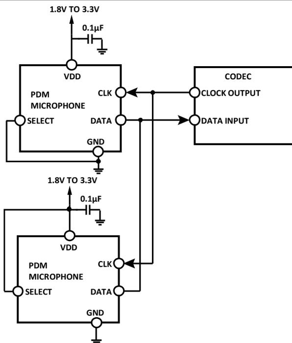
Figure 11. Stereo PDM Microphone Connection to Codec
