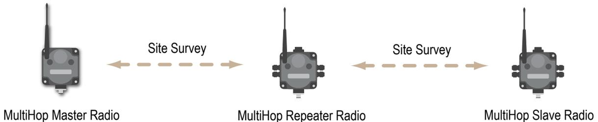
After MultiHop radios are communicating to their parents, the network formation information is transmitted back to the radio master, creating a path that is stored in each parent radio's routing tables. Each parent radio stores only one link or step along a path to an end radio. The routing information for non-MultiHop Modbus slave devices is stored as the devices are accessed by the host system.
