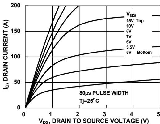
Figure 9. Saturation Characteristics
