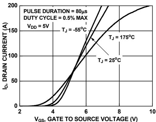
Figure 7. Transfer Characteristics
