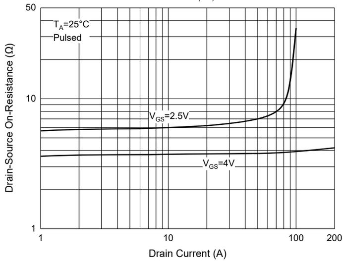
Fig. 4 -  $R_{DS(ON)} - V_{GS}$
