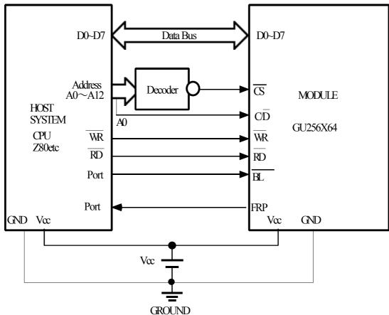
CAUTION: Because of adoption of C-MOS input logic in the module, shorter than 30cm cable length between a host system and the module is kindly suggested for free from permanent damages caused by noise.
