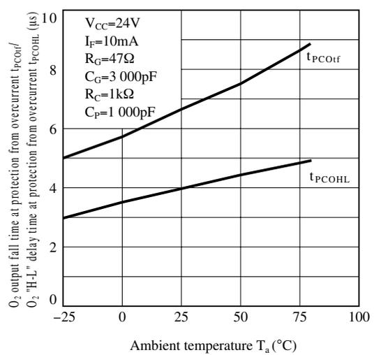
**Fig.33 Error Signal "High-Low" Propagation Delay Time vs. Ambient Temperature**
