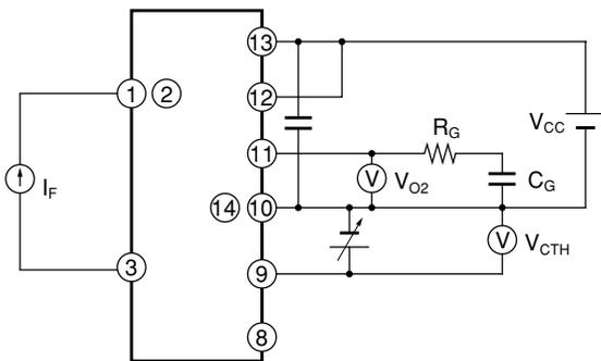
**Fig.10 Test Circuit for O<sub>2</sub> Output Voltage at Overcurrent Protection**
