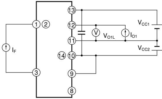
**Fig.2 Test Circuit for O<sub>2</sub> High Level Output Voltage**
