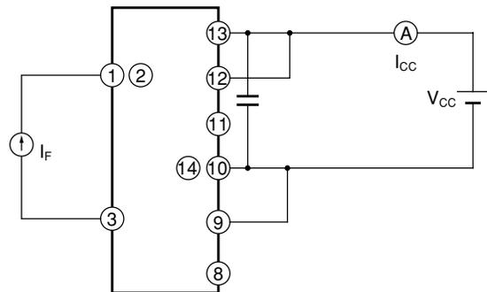
**Fig.7 Test Circuit for Instantaneous Common Mode Rejection Voltage**
