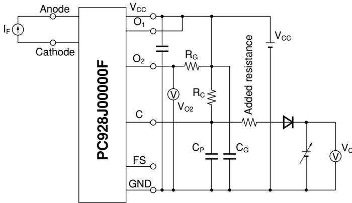
**Fig.40 Example of The Application Circuit (IGBT Drive for Inverter)**
