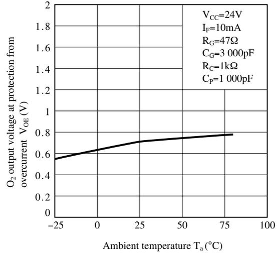
**Fig.35 Low Level Error Signal Voltage vs. Ambient Temperature**
