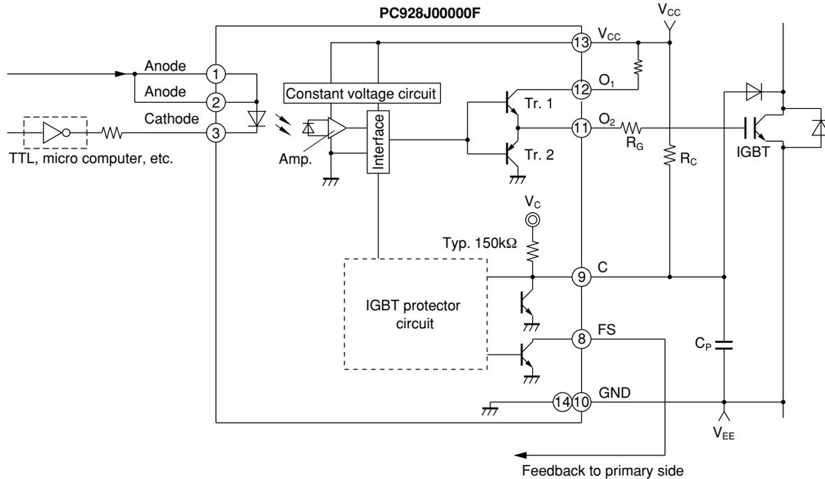
1. Detection of increase in  $V_{CE(sat)}$  of IGBT due to overcurrent by means of C terminal (pin ⑨)
