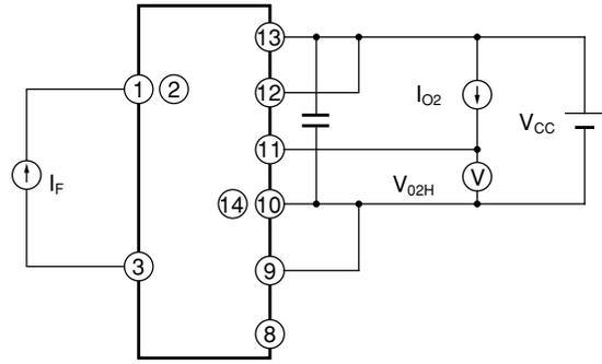
**Fig.3 Test Circuit for O<sub>2</sub> Low Level Output Voltage**
