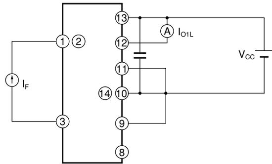
**Fig.5 Test Circuit for "Low→High" Input Threshold Current**
