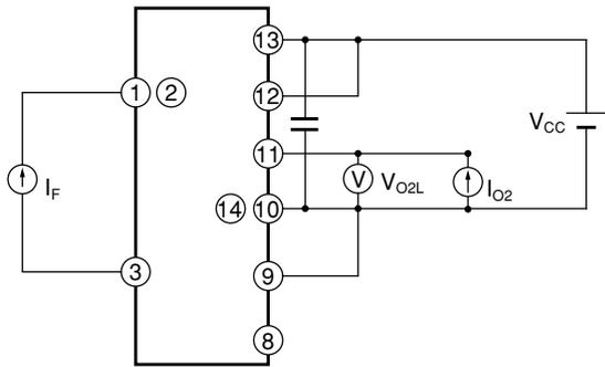
**Fig.4 Test Circuit for O<sub>1</sub> Leak Current**
