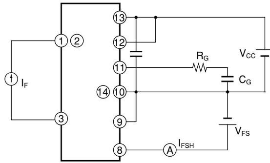
**Fig.13 Test Circuit for O<sub>2</sub> "High→Low" Propagation Delay Time at Overcurrent Protection, O<sub>2</sub> Fall Time at Overcurrent Protection**
