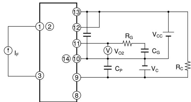
**Fig.11 Test Circuit for O<sub>1</sub> Low Level Error Signal Voltage**
