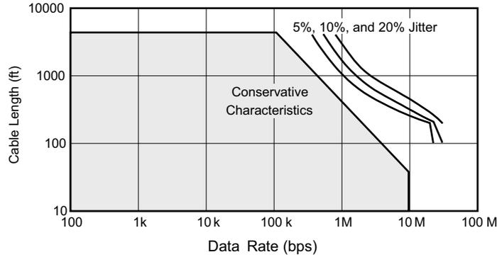
**Figure 9-2. Cable Length vs Data Rate Characteristic**
