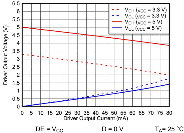
**Figure 6-1. Driver Output Voltage vs Driver Output Current**
