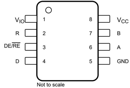
**Figure 5-2. THVD1439V, THVD1449V, 8-Pin (SOIC), Top View**
