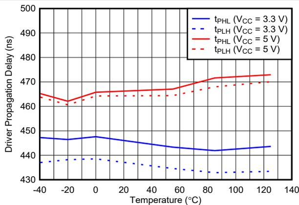
**Figure 6-5. THVD1439, THVD1439V Driver Propagation Delay vs Temperature**
