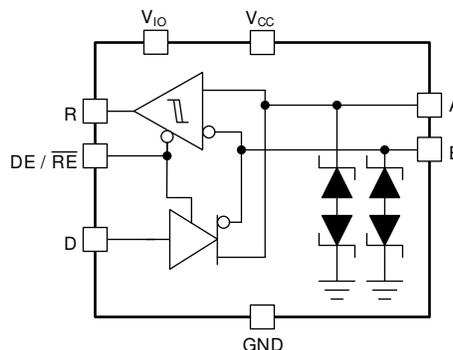
Figure 8-2. THVD1439V and THVD1449V Block Diagram
