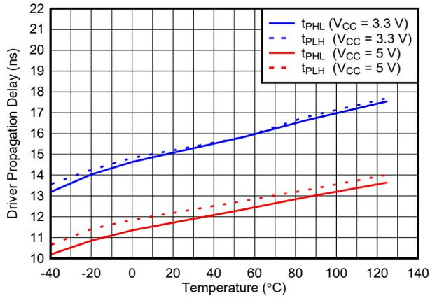
**Figure 6-7. THVD1449, THVD1449V Driver Propagation Delay vs Temperature**
