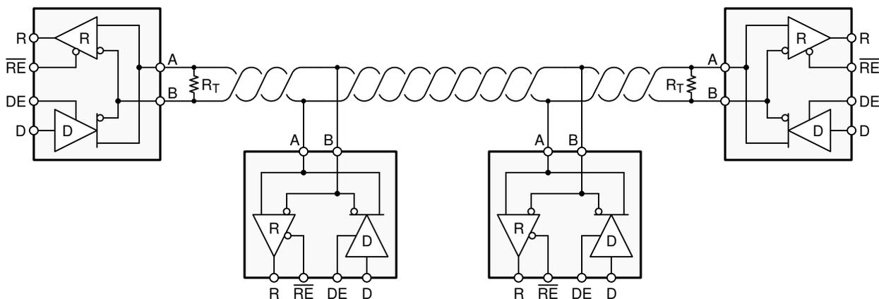
**Figure 9-1. Typical RS-485 Network With Half-Duplex Transceivers**
