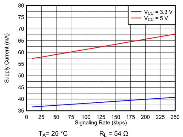
**Figure 6-6. THVD1439, THVD1439V Supply Current vs Signal Rate**
