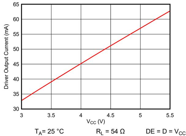
**Figure 6-3. Driver Output Current vs Supply Voltage**
