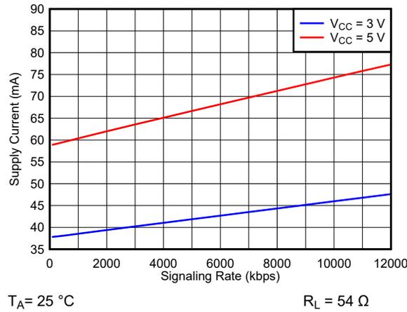
**Figure 6-9. THVD1449, THVD1449V Supply Current vs Signal Rate**
