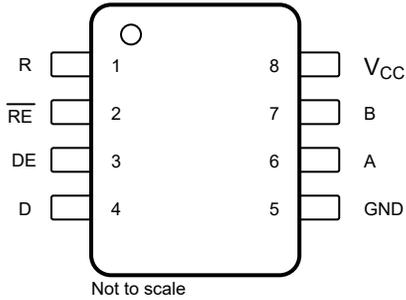
**Figure 5-1. THVD1439, THVD1449, 8-Pin (SOIC), Top View**
