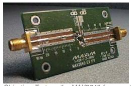
Objective: To tune the MAX2640 for operation at 345MHz for wireless security-system transmission.
