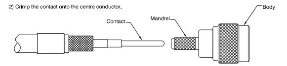
3) Insert the contact into the body and ensure that it captivates. Make sure that the braid is on the outside of the mandrel. Slide the ferrule over the braid until the ferrule butts up against the body. Crimp the ferrule using the correct tool for the connector.
