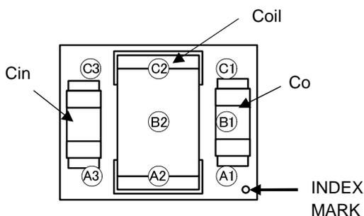
Figure 2. Pin Configuration(s)
