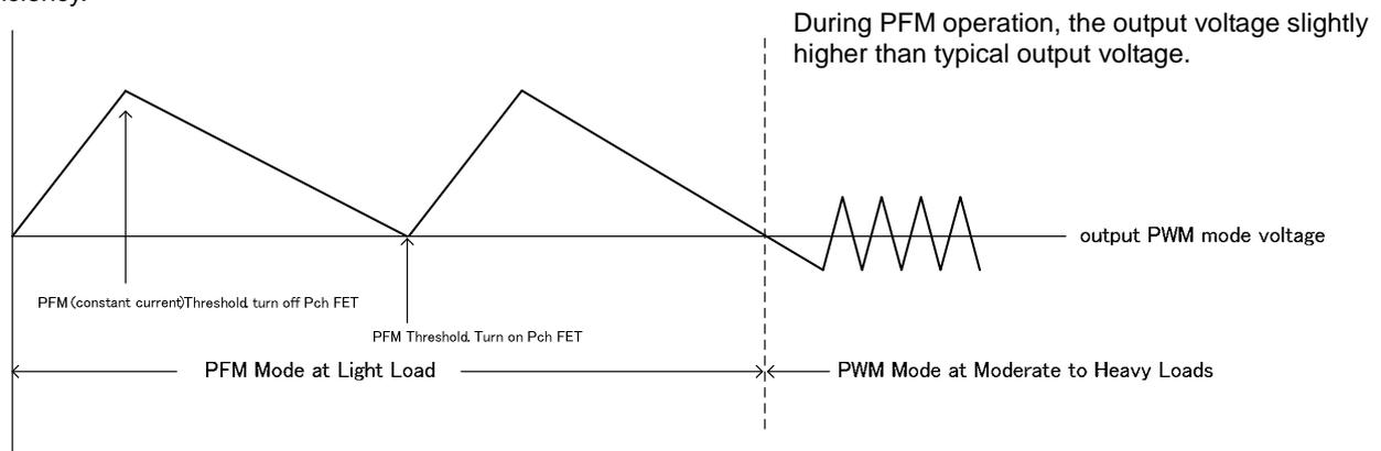
Figure 4. Operation of PFM mode and PWM mode
