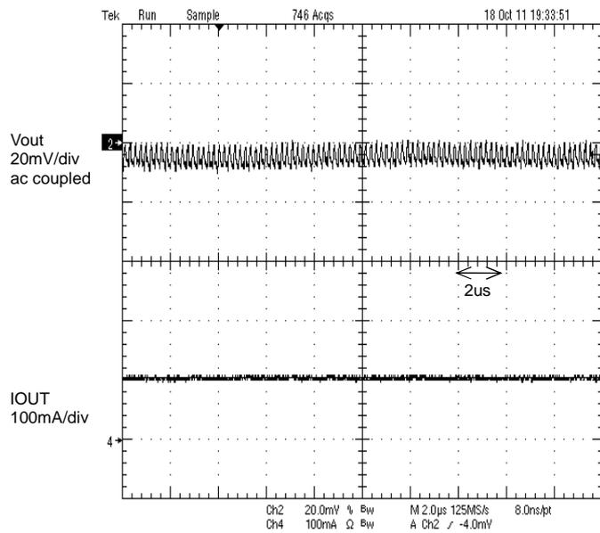
Figure 12. PWM mode Operation
