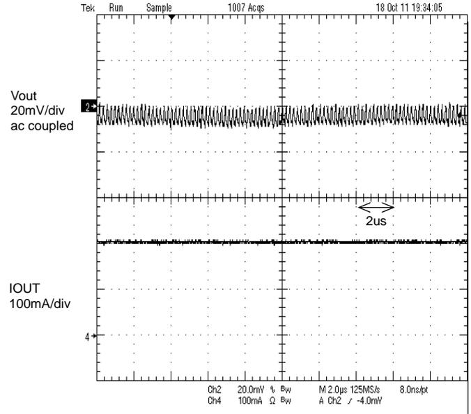
Figure 14. PWM mode Operation
