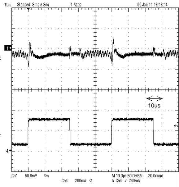
Figure 8. Load transient response 50mA to 350mA
