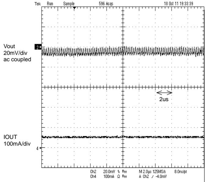
Figure 10. PWM mode Operation
