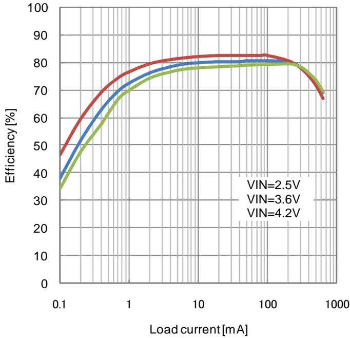
Figure 17. Efficiency vs Load current
