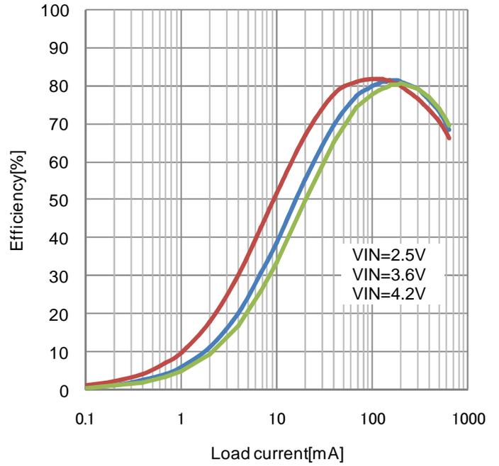
Figure 34. Efficiency vs Load current
