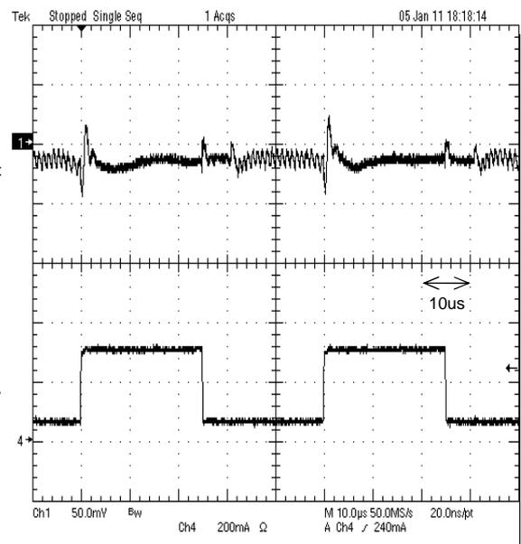
Figure 24. Load transient response 50mA to 350mA
