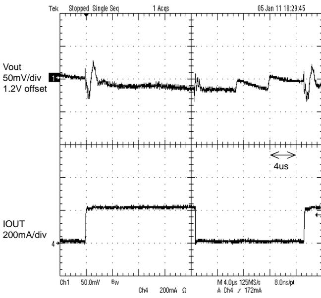
Figure 23. Load transient response 5mA to 200mA
