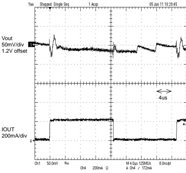
Figure 7. Load transient response 5mA to 200mA
